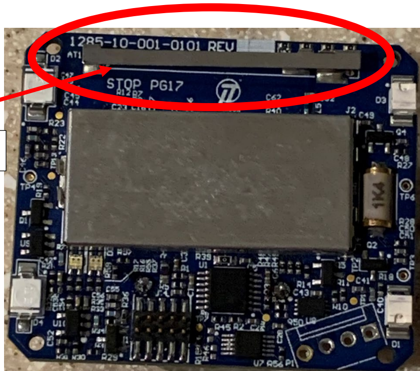
BLUband V3 Showing Antenna Location
