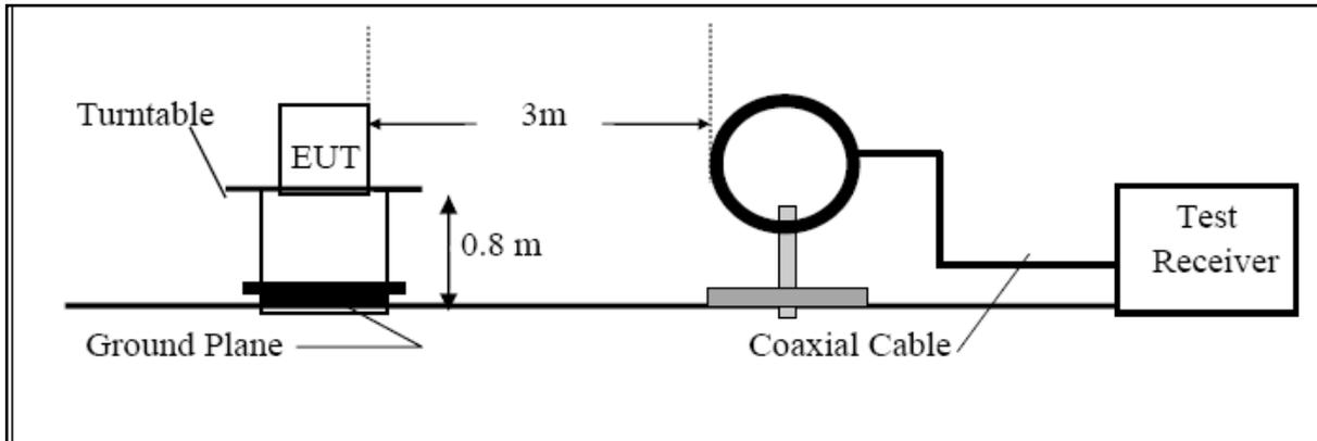
For Radiated Emission 30~1000MHz
