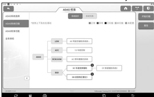
The ADAS system supports two display modes: topology and list. Click [Start Scanning] to scan the ADAS system one by one. After the scan is complete, click the system displayed in red (the system is displayed in red, indicating that there is a fault code in the system) to view the fault code, and click the system that works normally (the system is displayed in green, indicating that the system works normally) to perform other diagnostic functions.
