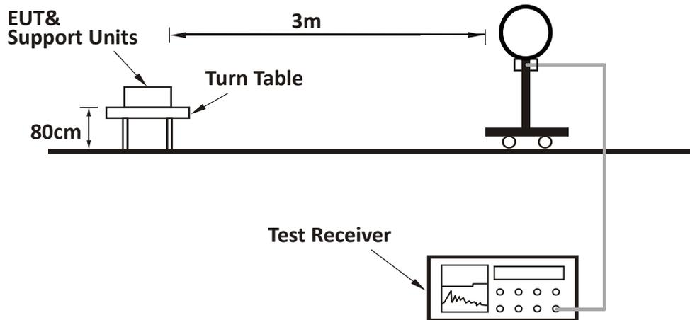
For Radiated emission 30MHz to 1GHz:
