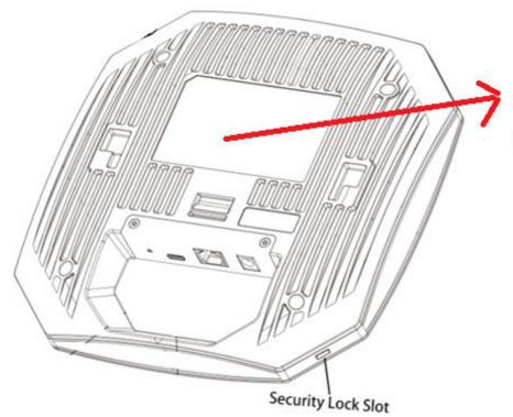
The label will be attached here on the bottom of the AP.
