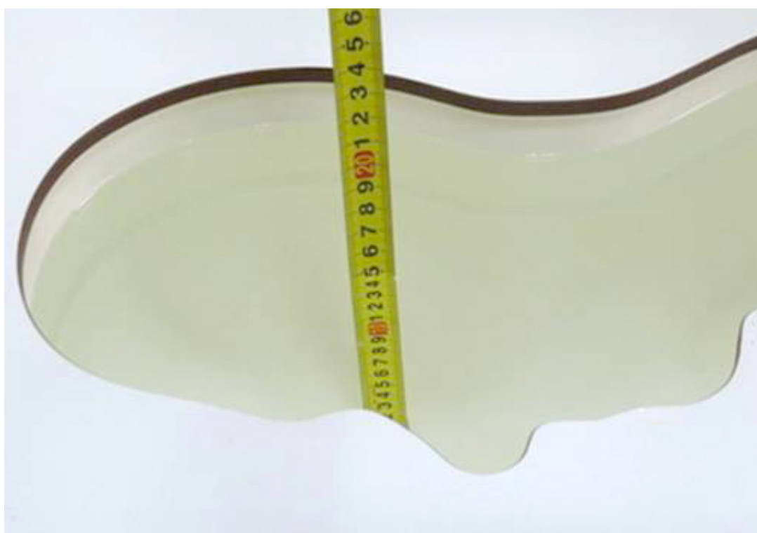
Liquid depth in the head Phantom (2600 MHz, 15.4cm depth)
