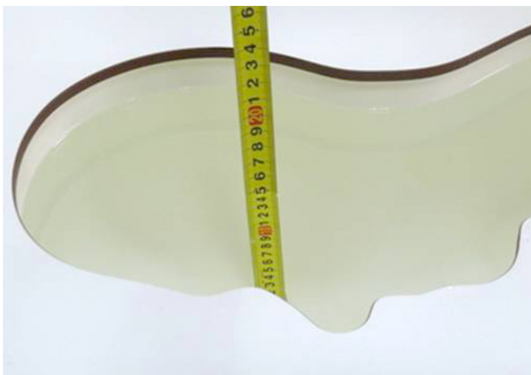
Liquid depth in the head Phantom (2450 MHz, 15.4cm depth)
