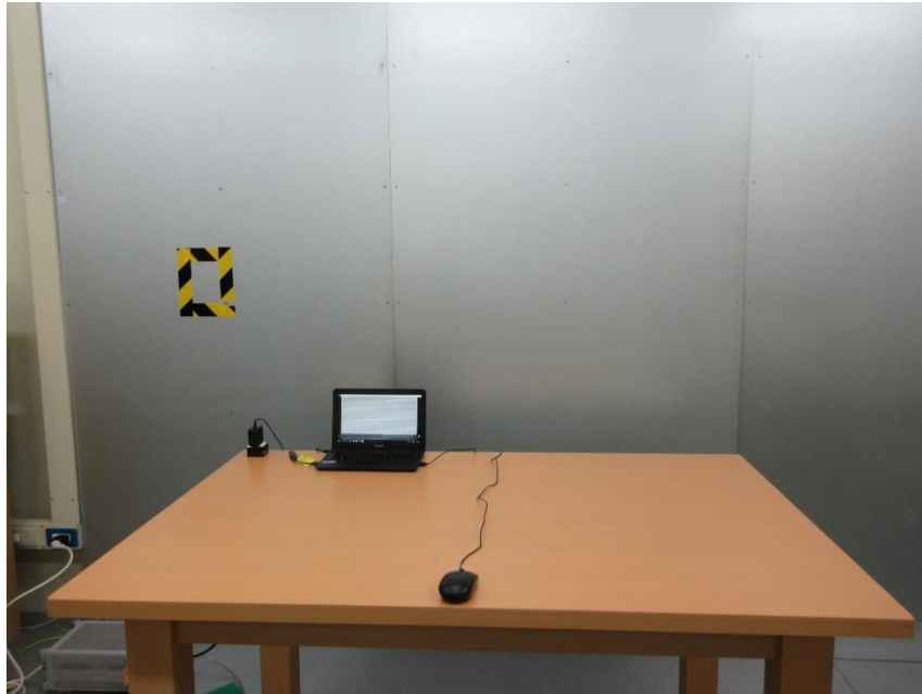
Photograph 1: Set-up for Conducted Emission (AC Mains)
