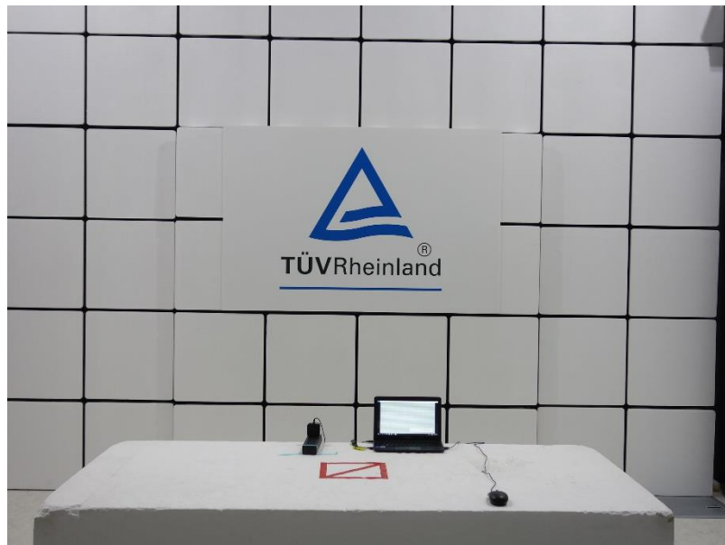
Photograph 2: Set-up for Radiated Emission (up to 1 GHz)
