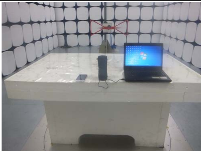
Radiated Spurious Emissions Test Setup Below 1GHz
