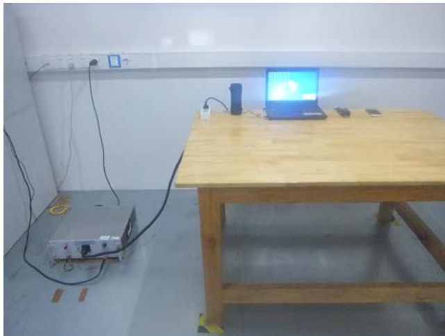
Conducted Emissions Test Setup Front View
