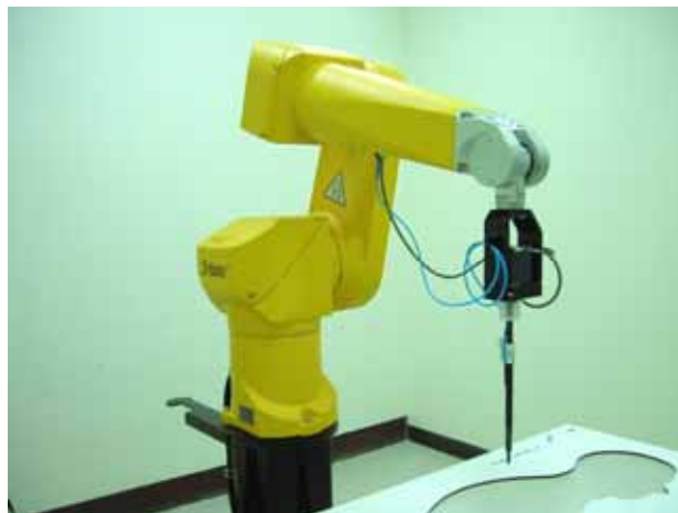
Fig. 5.2 Probe setup on robot
