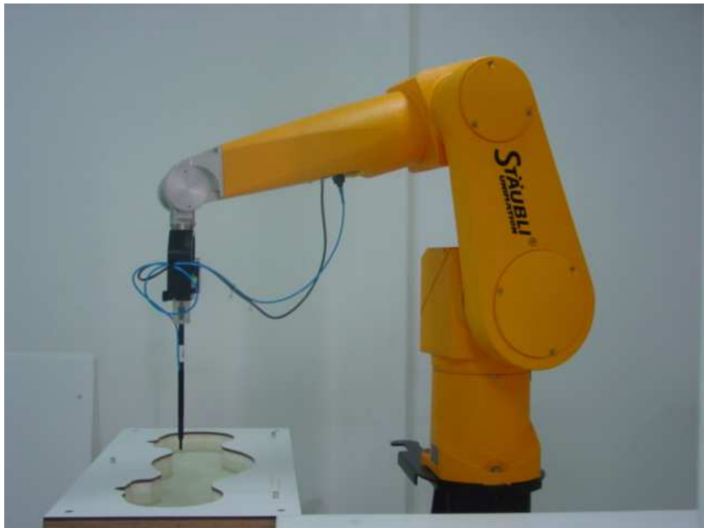
Picture B1: Specific Absorption Rate Test Layout
