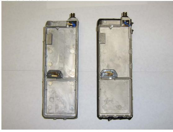
The following two photographs show the chassis with installed PC boards. As can be seen the internal design is unaltered. There is a difference in the shield cover arrangement. The new design features a single piece shield with improved grounding to the chassis. The result is a mechanical construction offering equal performance to the original design.
