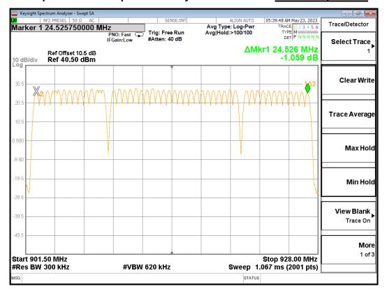
Screen Capture from the spectrum analyzer: 50 Channels FSK 28.8kbps Mode
