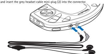
The headset lead functions as the antenna of the radio, so let it hang freely.
