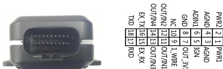
Figure 1. The 18-pin Connector on the GV600MG
