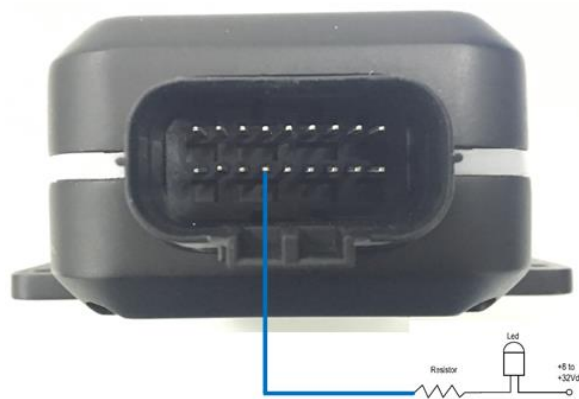
Figure 11. Typical Connection with a LED
