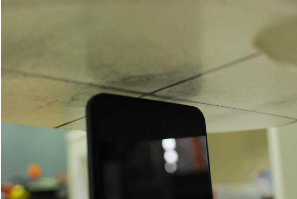
SAR Test Setup Photo 19 –Bottom Edge at 3 mm
