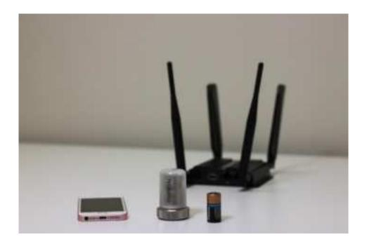
Connecting Vibration Motes to your WiFi network is a quick and simple process, which utilizes a technology called Blink Up. This is a method of using your mobile device to optically communicate WiFi login credentials to a Vibration Mote.
