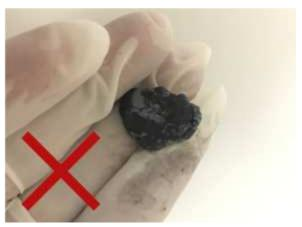
3.2 Roll epoxy into a 2-3 inch strip, then form a ring on the bottom of the Mote mount.
