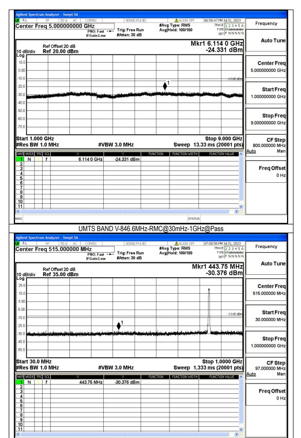
UMTS BAND V-846.6MHz-RMC@1GHz-9GHz@Pass
