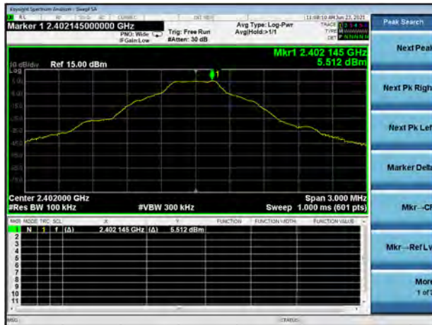
GFSK LOW CHANNEL, CARRIER LEVEL
