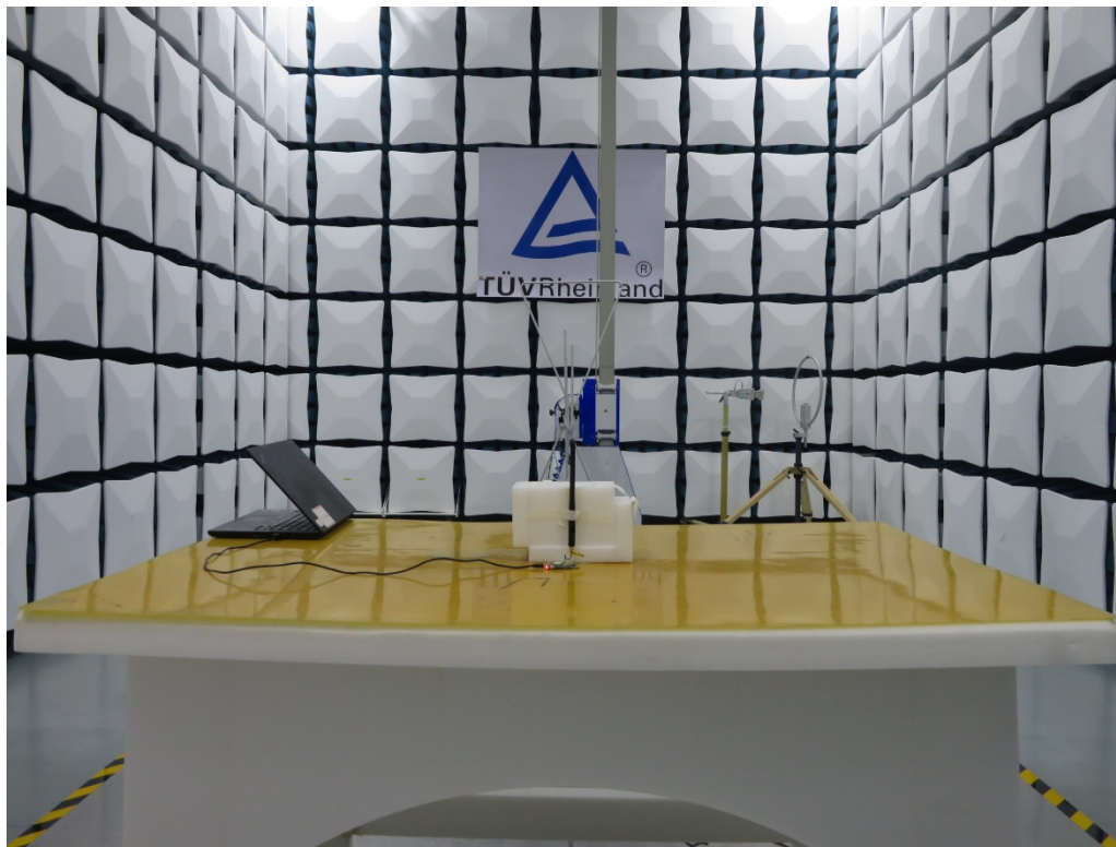
Photograph 1: Set-up for Radiated Spurious Emission, Below 1GHz
