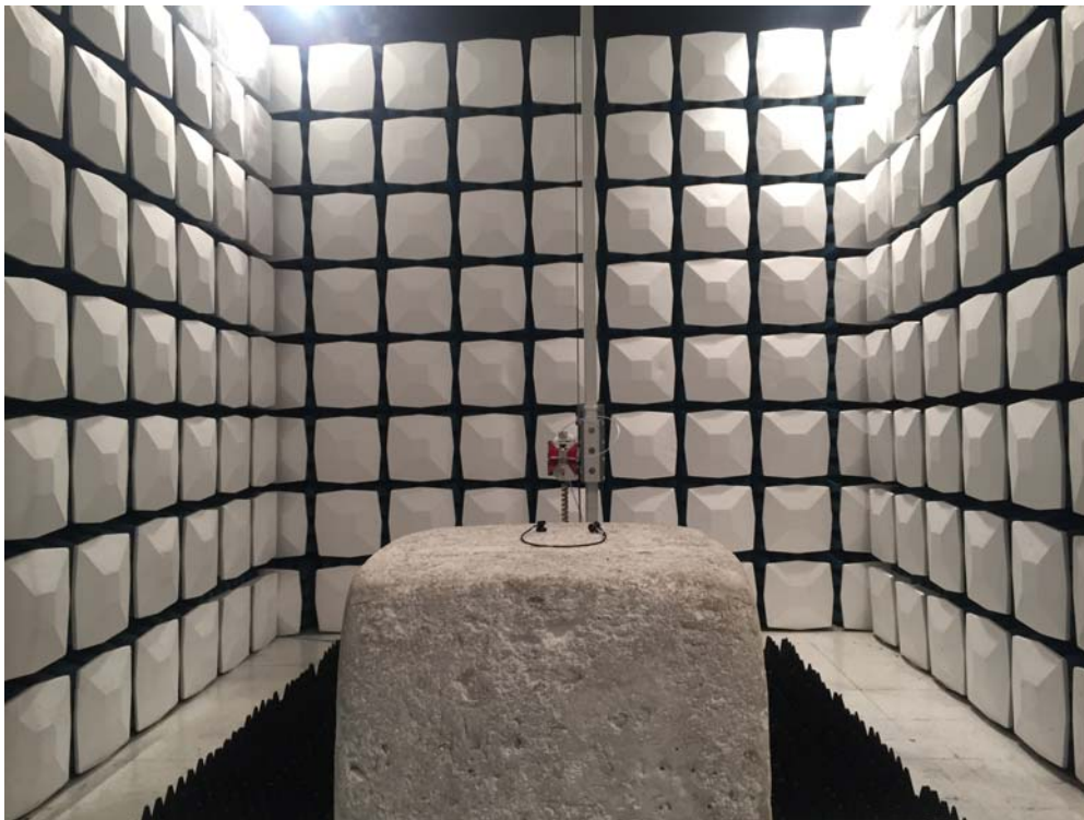
Description: Radiated Emission Test Setup for 1~18GHz
