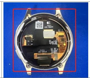
The antenna is Metal frame antenna.
