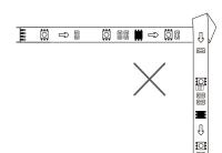
Recommended Tip: Try not to bend at electronic components like light beads, bonding pad to avoid short circuit.
