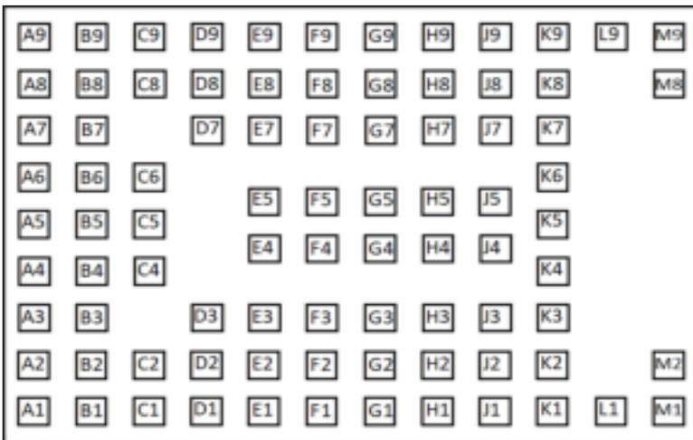
Figure 3: MAYA-W1 series pin assignment (top view)
