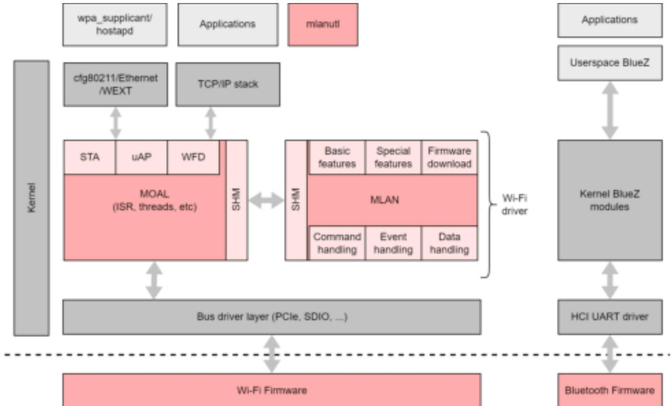
Figure 14: Basic Wi-Fi and Bluetooth driver architecture
