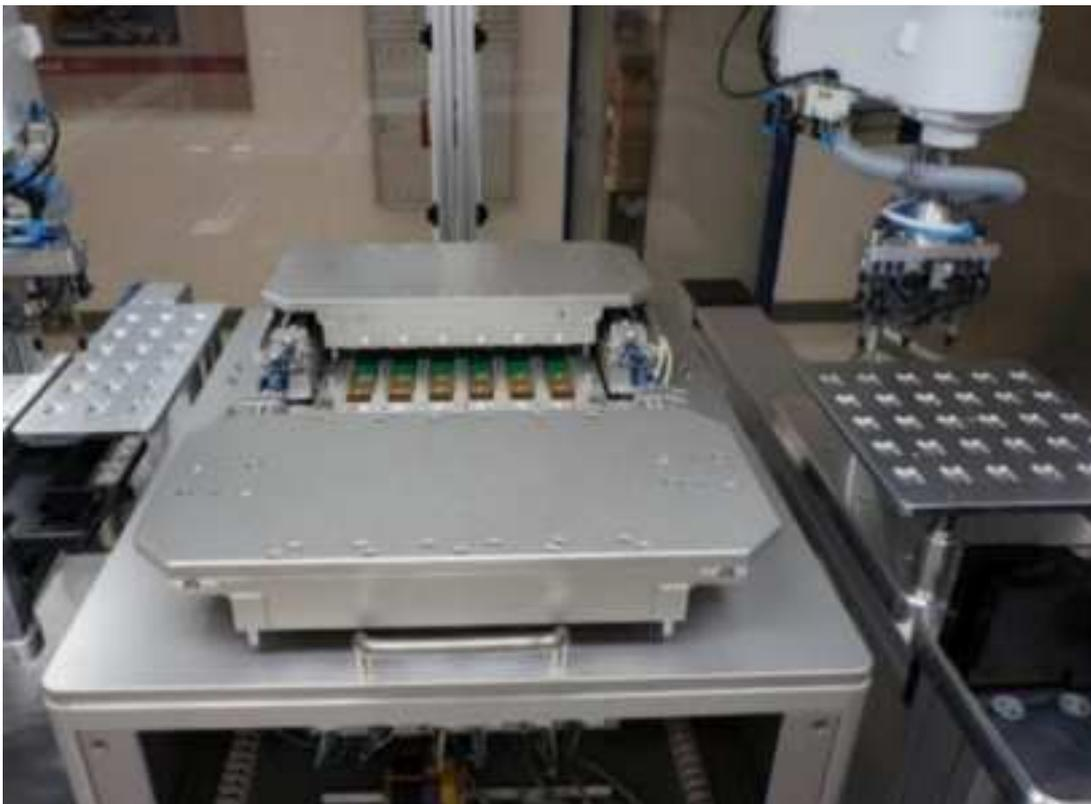
**Figure 17: Automatic test equipment for module test**
