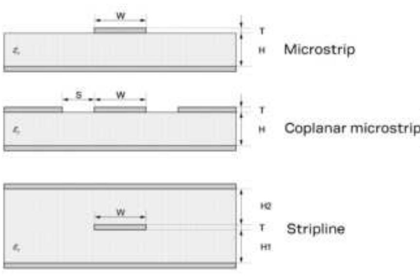
**Figure 8: Transmission line trace design**
