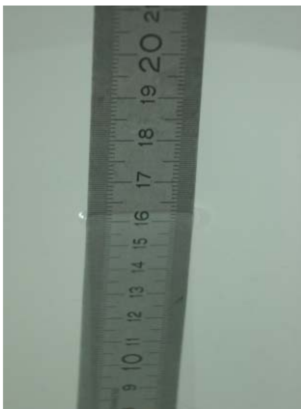
Fig. 37: Liquid depth for GPRS 1900 Body measurements.
