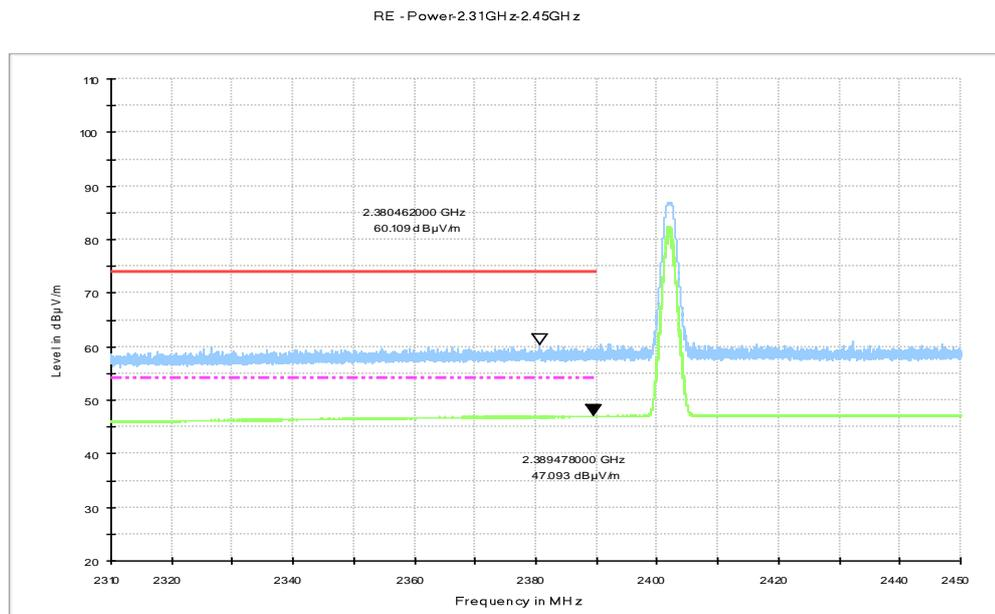
Fig.3. Frequency Band Edges: GFSK, 2402 MHz, 2.31 GHz – 2.45GHz
