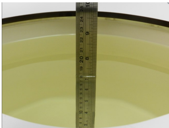
Fig 10.1 Photo of Liquid Height for Body SAR
