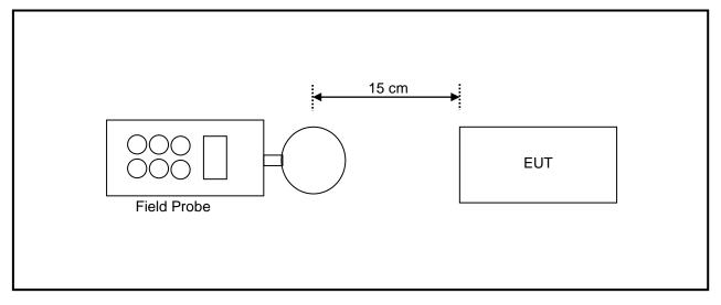
Note: Measurements should be made from all sides and the top of the primary/client pair, with the 15 cm measured from the center of the probe(s) to the edge of the device.
