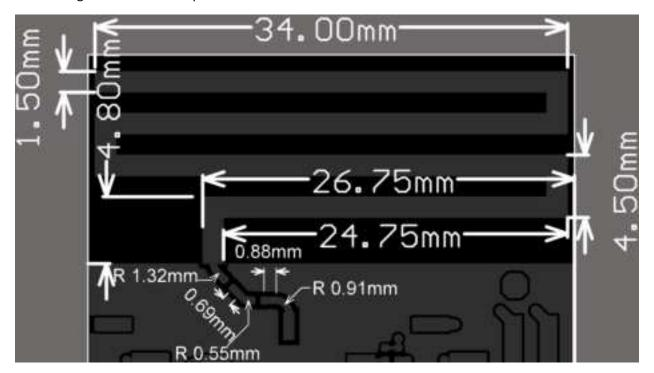
Below board shows the bottom layer layout of the reference board directly beneath the RF traces
