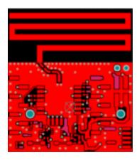
The figure below shows the Top layer layout of the reference host Sensor board focussed on RF traces and PCB antenna. The snapshot also indicates the critical dimensions that are required to be replicated in the design to maintain compliance.
