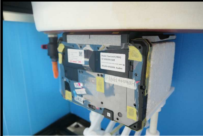
Bottom of Laptop Tested at 0 mm
