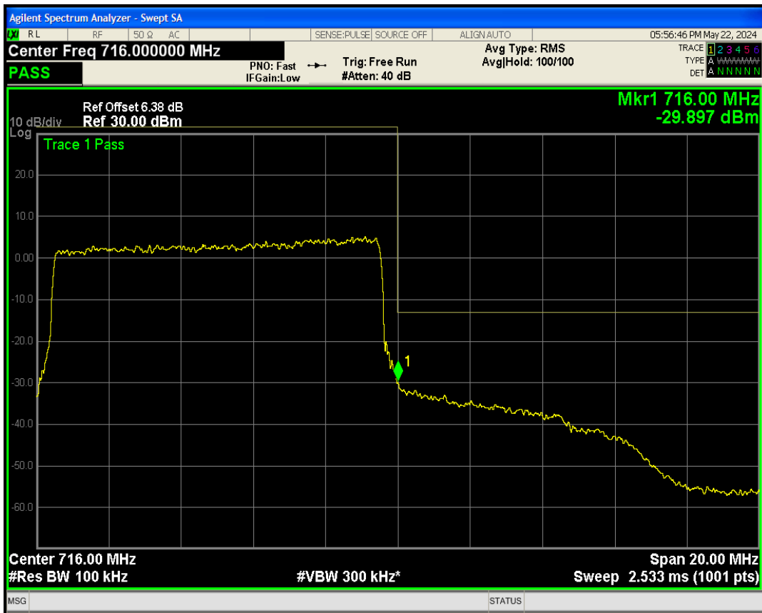
Band17 QAM16 BW=10MHz Channel=23800 RB Size=50 Position=#0
