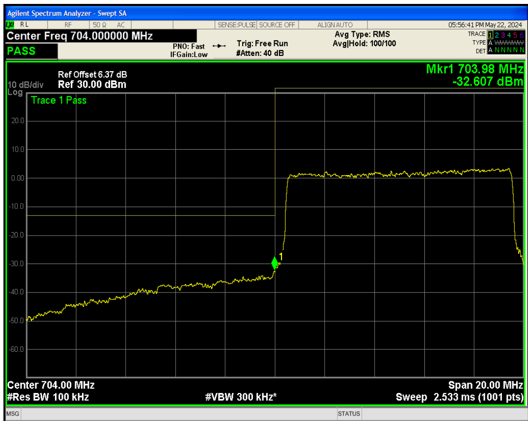
Band17 QPSK BW=10MHz Channel=23800 RB Size=50 Position=#0
