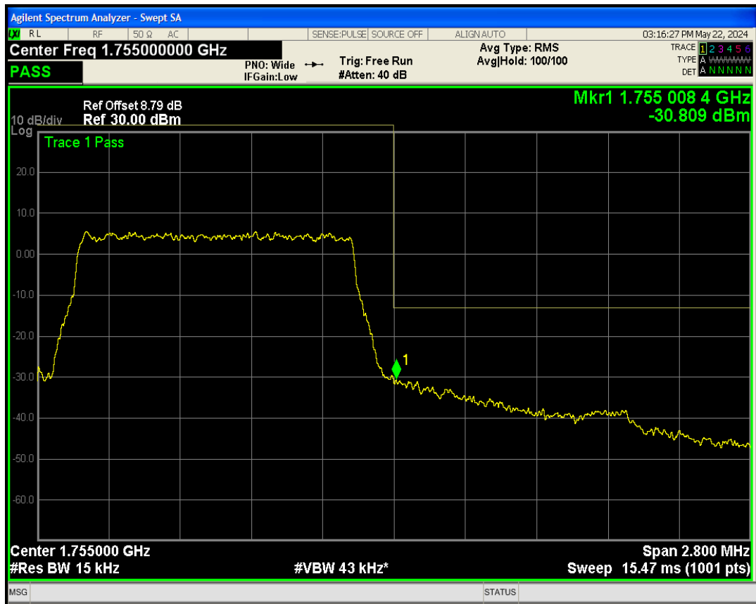
Band4 QAM16 BW=1.4MHz Channel=20393 RB Size=6 Position=#0
