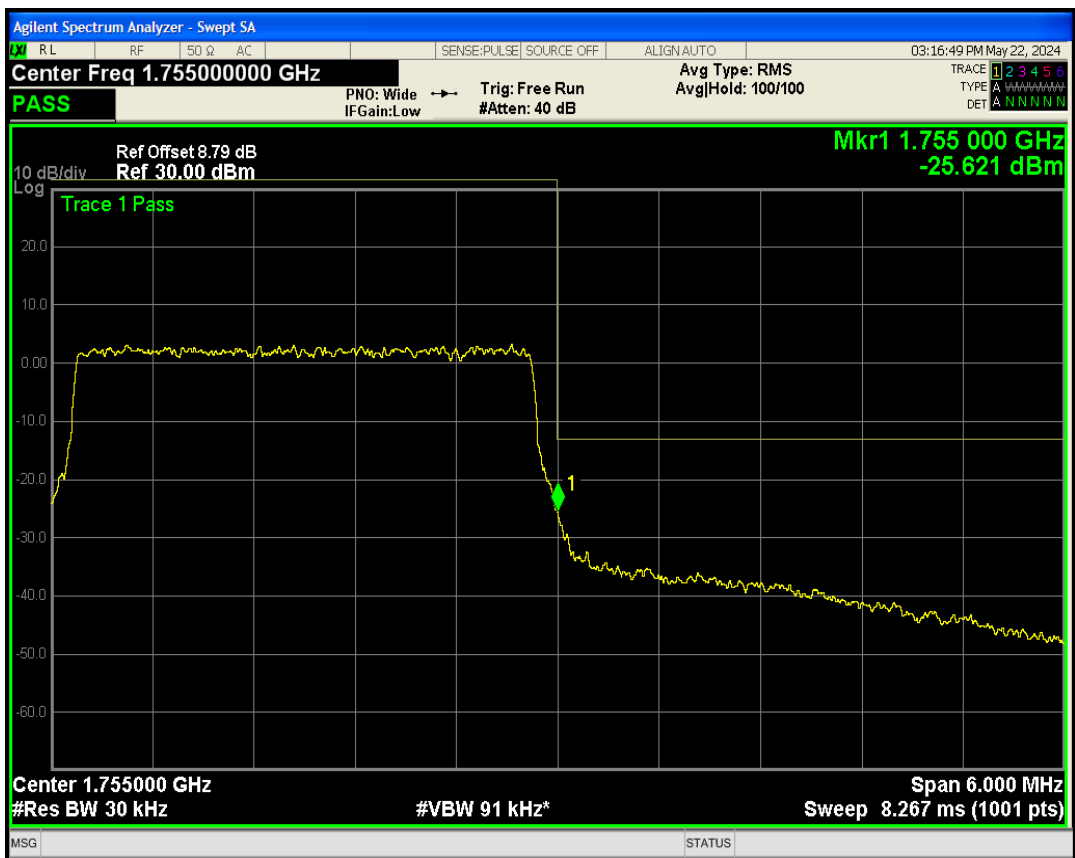
Band4 QPSK BW=5MHz Channel=19975 RB Size=25 Position=#0
