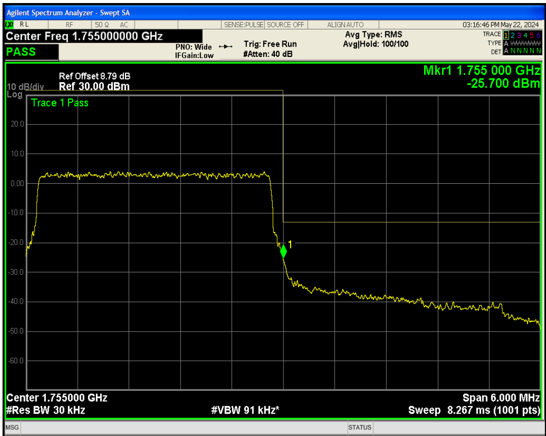
Band4 QAM16 BW=3MHz Channel=20385 RB Size=15 Position=#0
