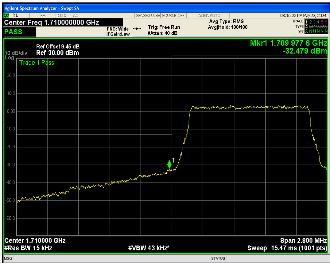
Band4 QPSK BW=1.4MHz Channel=20393 RB Size=6 Position=#0
