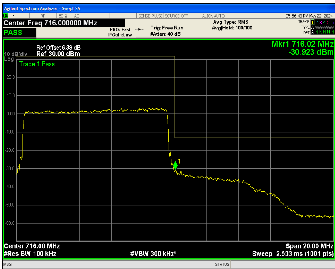
Band2 QPSK BW=1.4MHz Channel=18607 RB Size=6 Position=#0
