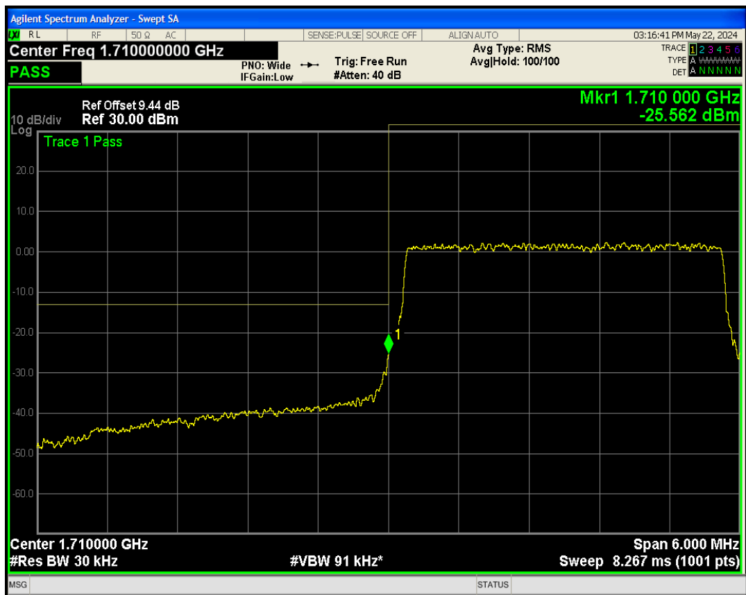
Band4 QPSK BW=3MHz Channel=20385 RB Size=15 Position=#0
