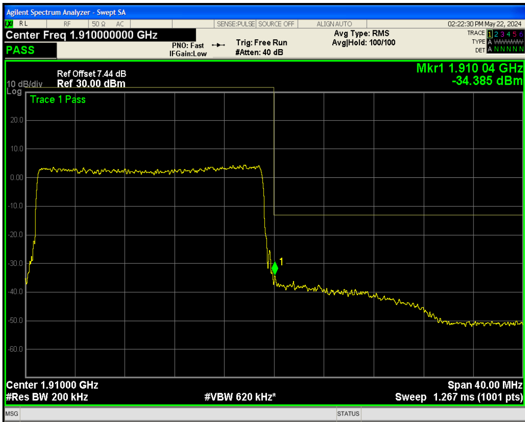
Band2 QAM16 BW=20MHz Channel=19100 RB Size=100 Position=#0
