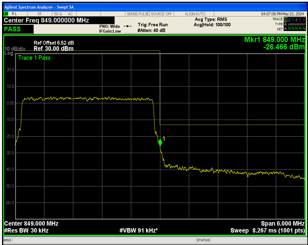
Band5 QAM16 BW=3MHz Channel=20635 RB Size=15 Position=#0
