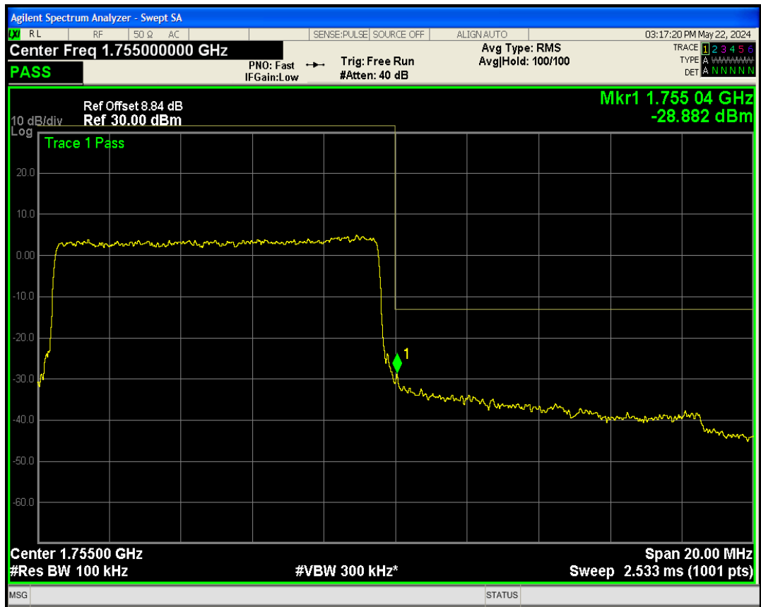
Band4 QAM16 BW=10MHz Channel=20350 RB Size=50 Position=#0
