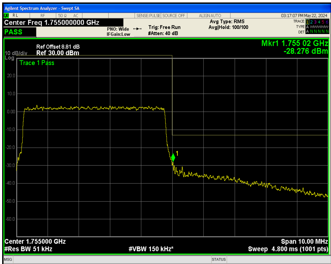
Band4 QPSK BW=10MHz Channel=20000 RB Size=50 Position=#0
