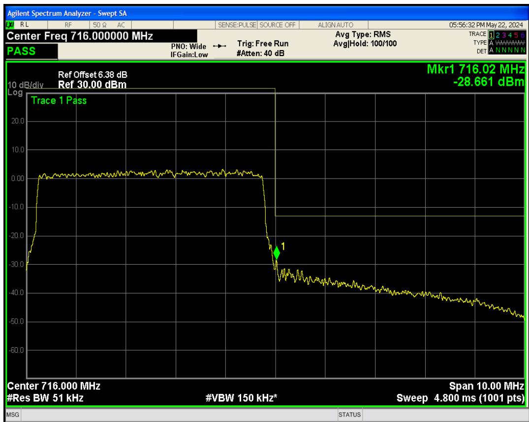
Band17 QPSK BW=10MHz Channel=23780 RB Size=50 Position=#0
