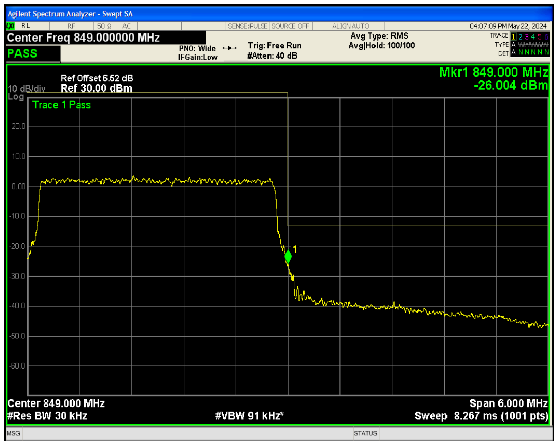
Band5 QPSK BW=5MHz Channel=20425 RB Size=25 Position=#0
