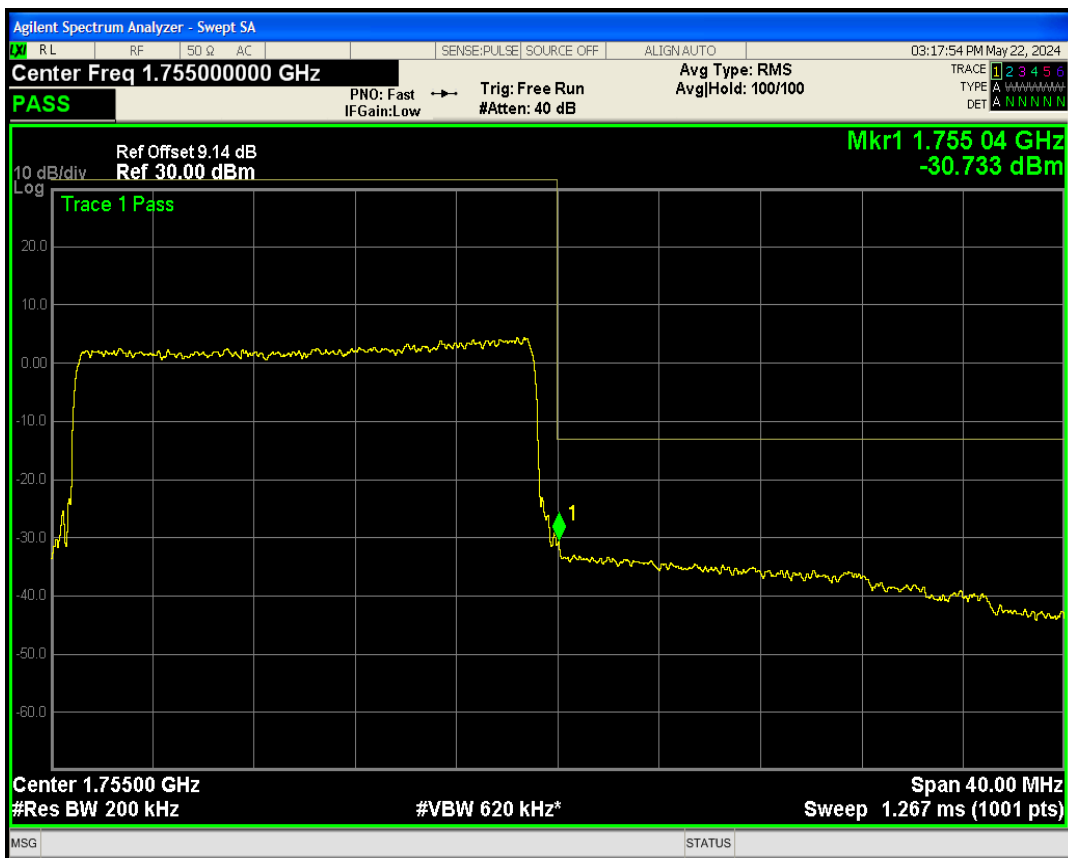
Band5 QPSK BW=1.4MHz Channel=20407 RB Size=6 Position=#0
