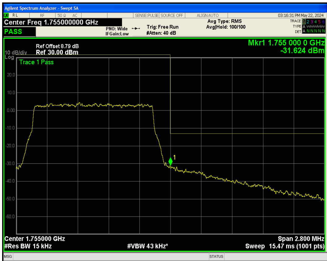
Band4 QPSK BW=3MHz Channel=19965 RB Size=15 Position=#0
