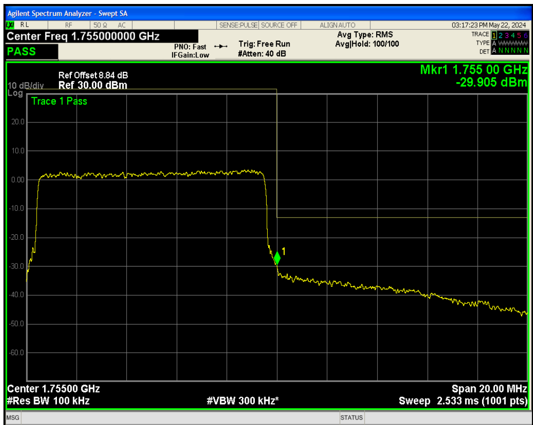
Band4 QPSK BW=15MHz Channel=20025 RB Size=75 Position=#0
