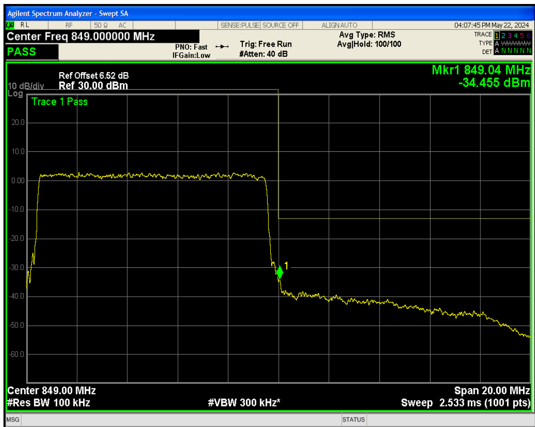
Band7 QPSK BW=5MHz Channel=20775 RB Size=25 Position=#0
