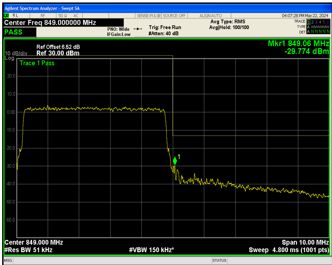
Band5 QPSK BW=10MHz Channel=20450 RB Size=50 Position=#0
