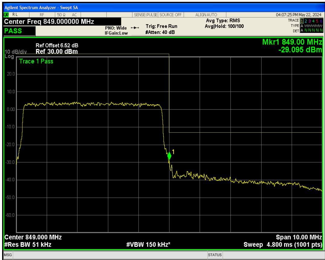
Band5 QAM16 BW=5MHz Channel=20625 RB Size=25 Position=#0
