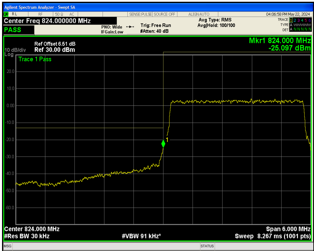
Band5 QAM16 BW=3MHz Channel=20415 RB Size=15 Position=#0
