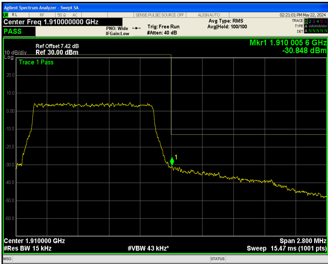
Band2 QAM16 BW=1.4MHz Channel=19193 RB Size=6 Position=#0
