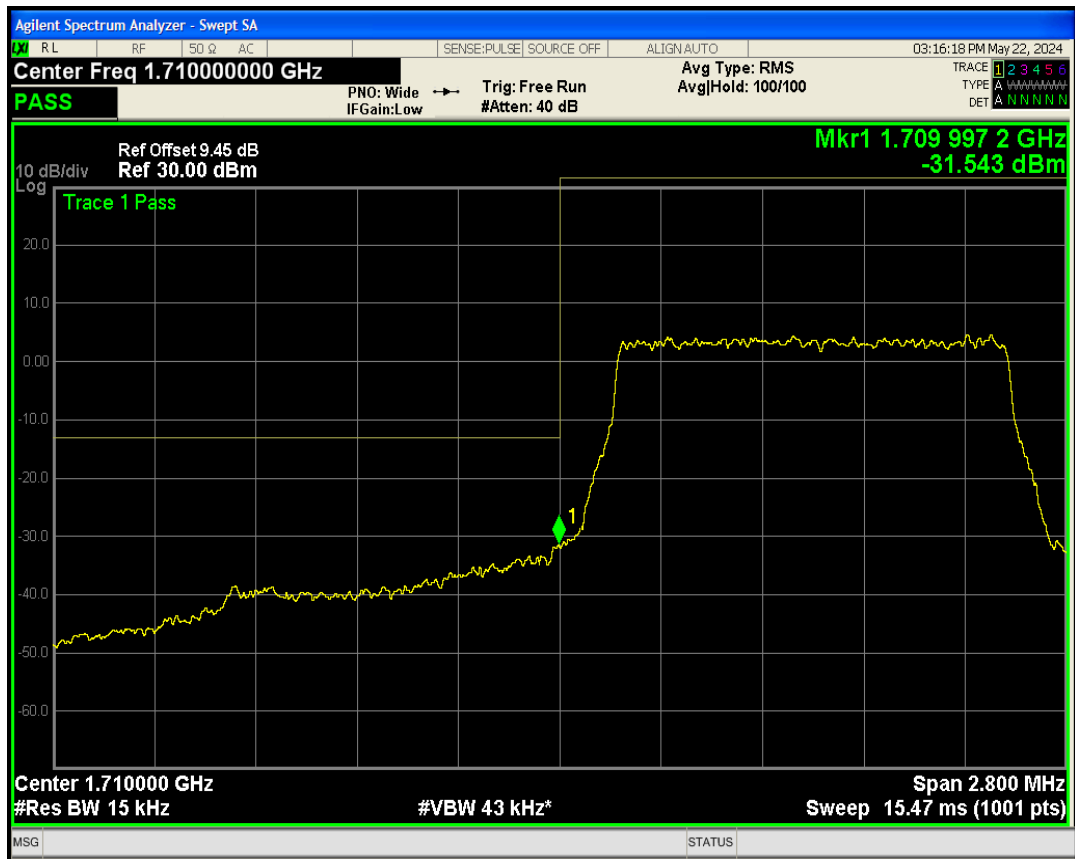
Band4 QAM16 BW=1.4MHz Channel=19957 RB Size=6 Position=#0
