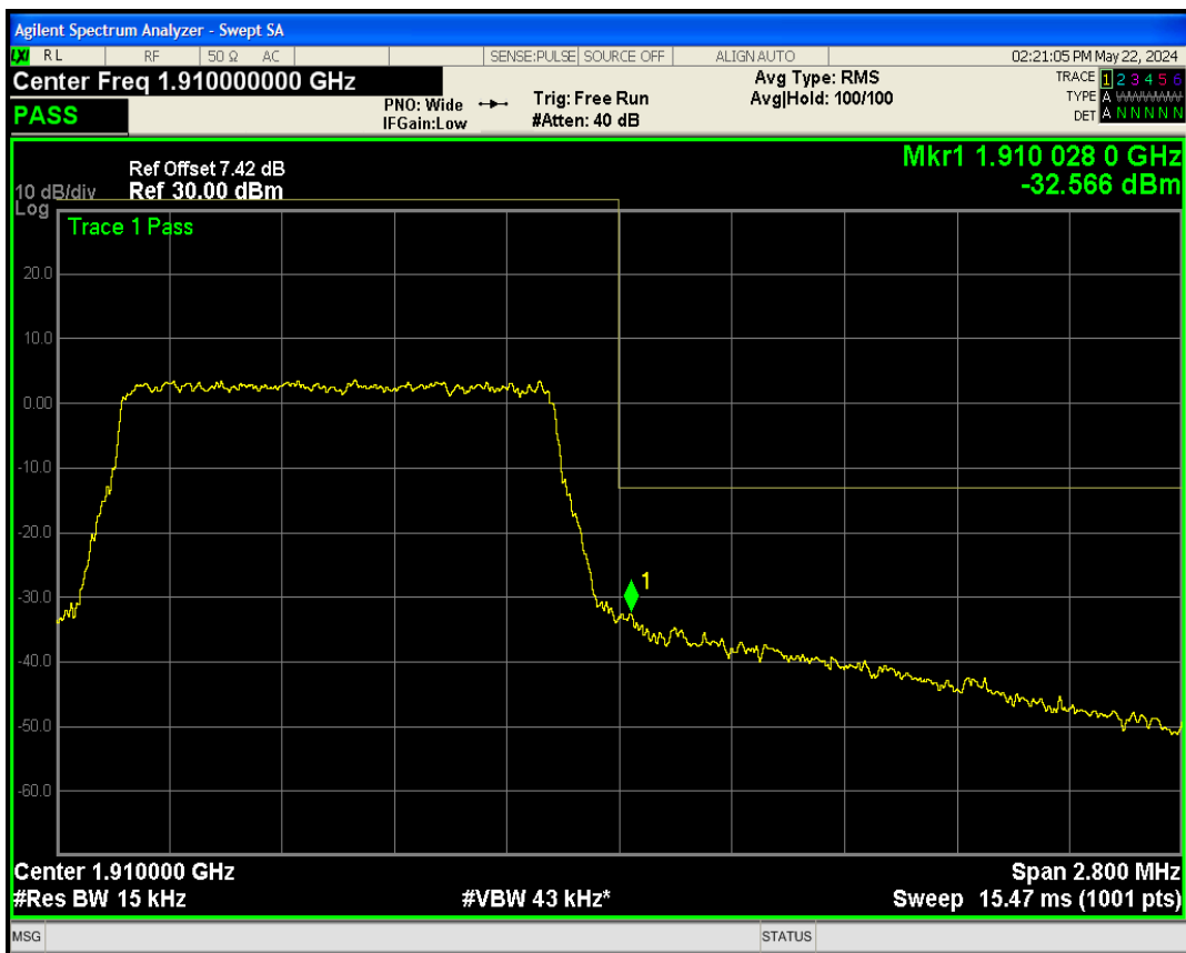
Band2 QPSK BW=3MHz Channel=18615 RB Size=15 Position=#0
