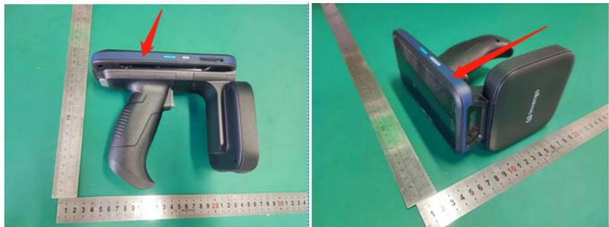
Picture 3: XC2908-G、XC2908-M、XC2908-BM、XC-RH500、XC-BM500、XC9915 , Thick glue front shell, slightly thicker
