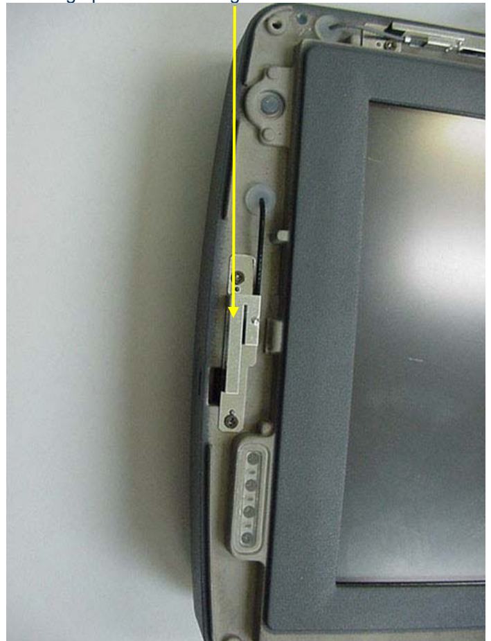
Photograph A.1-6 - Left Edge Bluetooth Antenna Location
