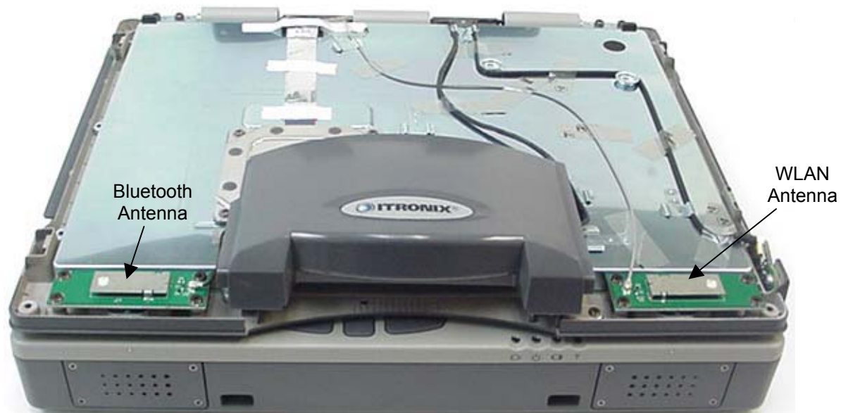
Photograph A-7 – Surface Mount Antenna Placement
