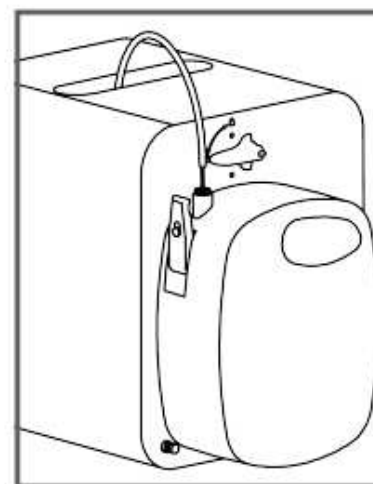
14. Insert the filament into the white guiding tube.
