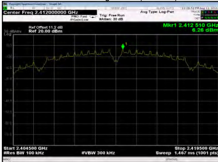
802.11b PSD for Bandedge Limit(CH-High)
