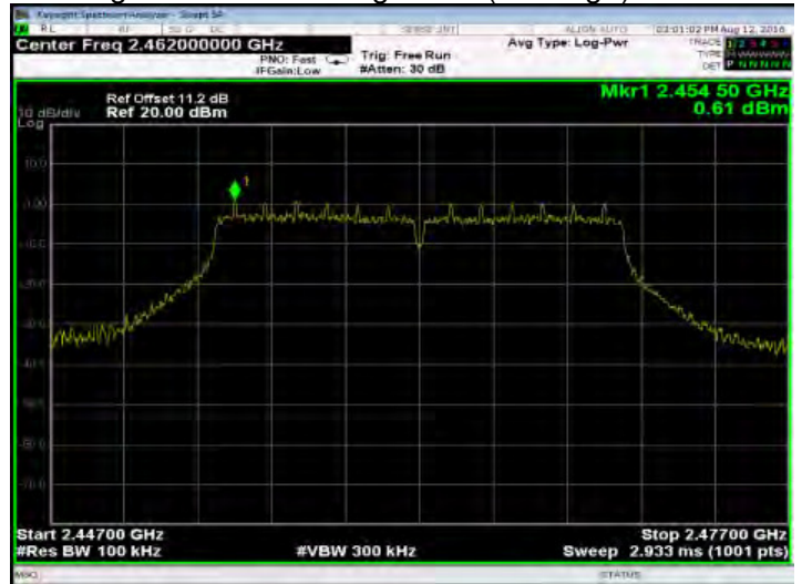
802.11n_HT20 PSD for Bandedge Limit(CH-Low)
