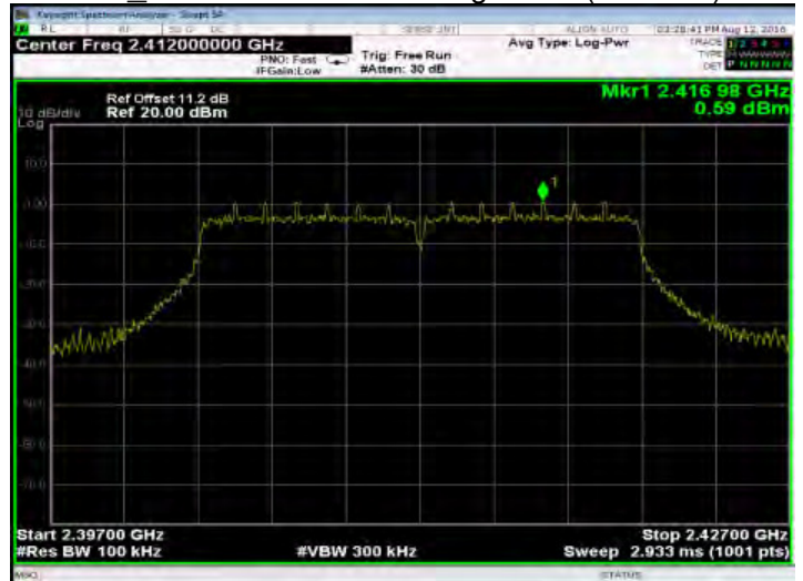
802.11n_HT20 PSD for Bandedge Limit(CH-High)
