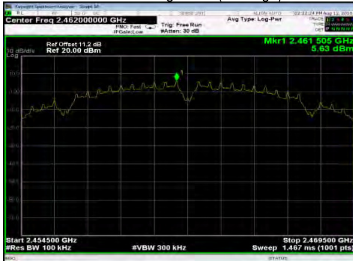
802.11g PSD for Bandedge Limit(CH-Low)
