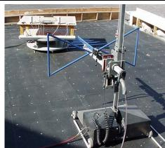
Photograph G-4 - 3115 Horn with LNA/Filter @ 3m
