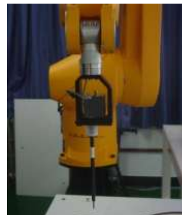
Picture C.3 E-field Probe
