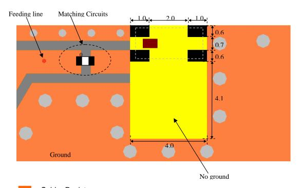
Solder Resist \*Line width should be designed to match  $50\Omega$  characteristic impedance, depending on PCB material and thickness.
