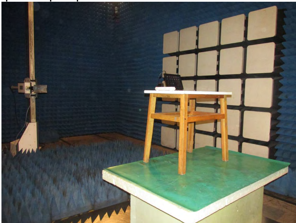
Photograph 4: Set-up for Spurious Emissions for 1 - 18GHz
