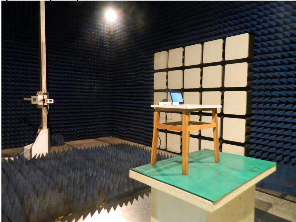
Photograph 5: Set-up for Spurious Emissions for 18 - 40GHz
