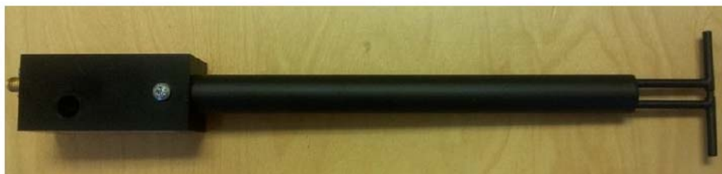
Figure 1 – MVG COMOSAR Validation Dipole
