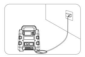
During charging, the micon on the screen of V4500 Plus will turn ON. If the charging rate reaches 18W or above, the icon will also turn ON.
