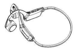
Press and hold the power button for 3 seconds. When the indicator light alternates between red and blue with a "power on" prompt tone, it indicates that the headphones have been successfully turned on.
