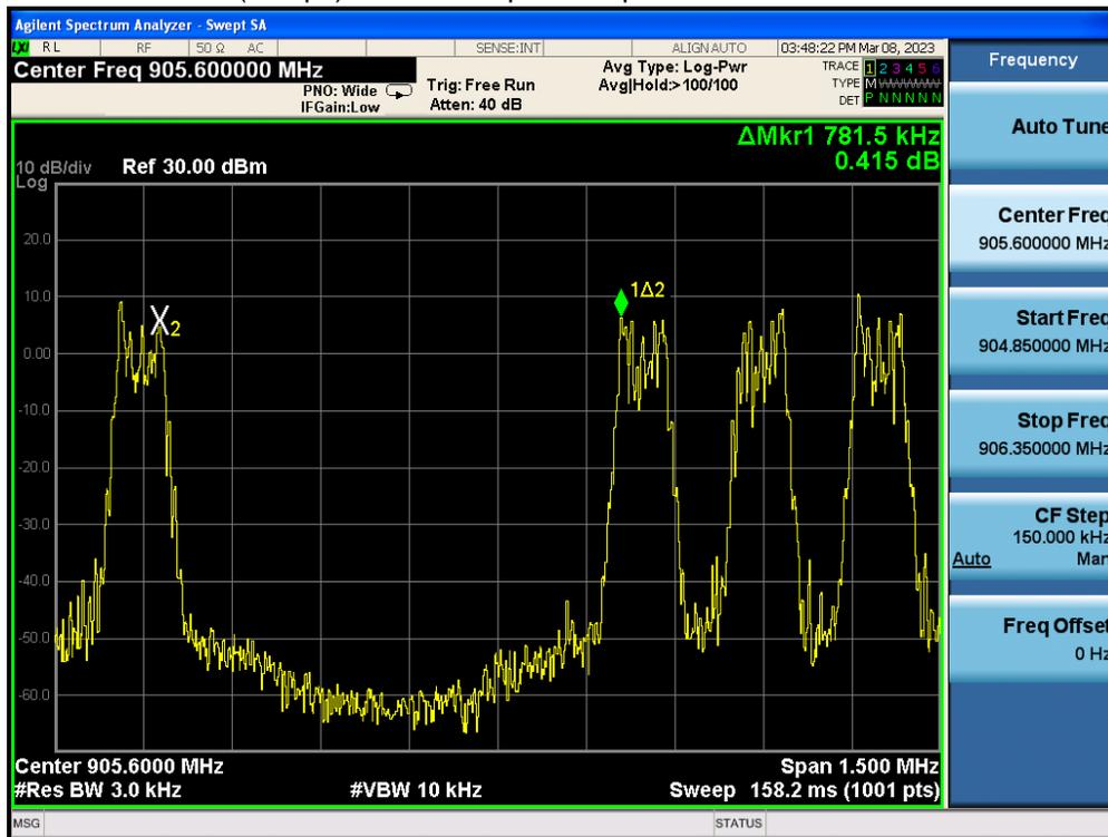
(1Mbps) Channel Separation plot on channel 52-53
