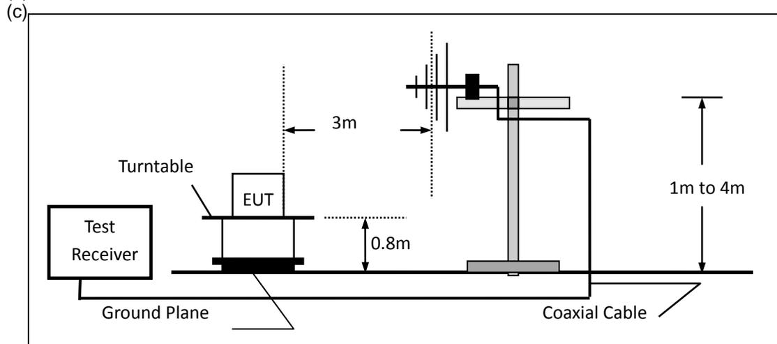
(c) For radiated emissions above 1000MHz
