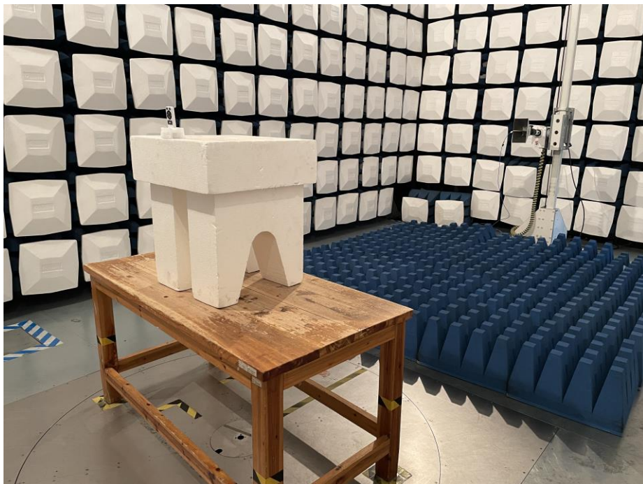
Test Setup For Radiated Emission (Above 1GHz)
