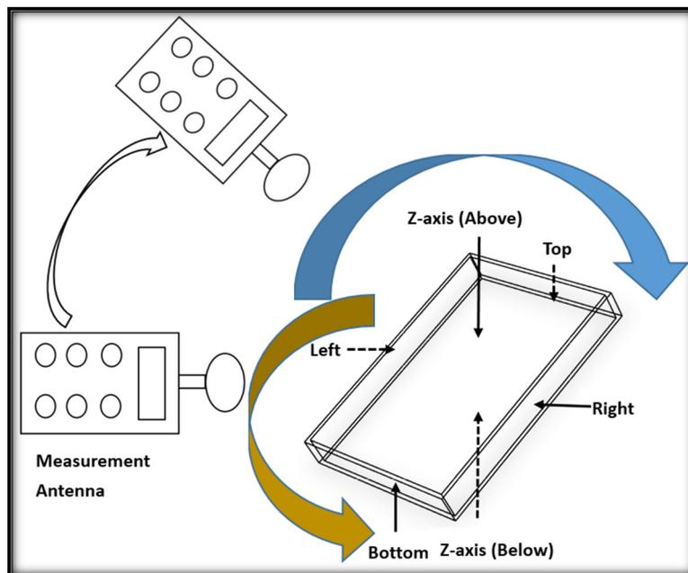
Note: The measurement antenna are move and surrounding the EUT when performed the test, the test results recorded the highest values for each sides of the EUT (left/right/top/bottom/z-axis)
