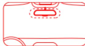
Note: Make sure to stick the electrostatic sticker on a flat and smooth part of the windshield, press it firmly, and avoid sticking it on the edge of the windshield's film to prevent it from falling down.
