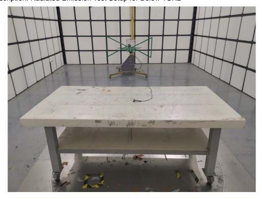
Description: Radiated Emission Test Setup for 1~18GHz
