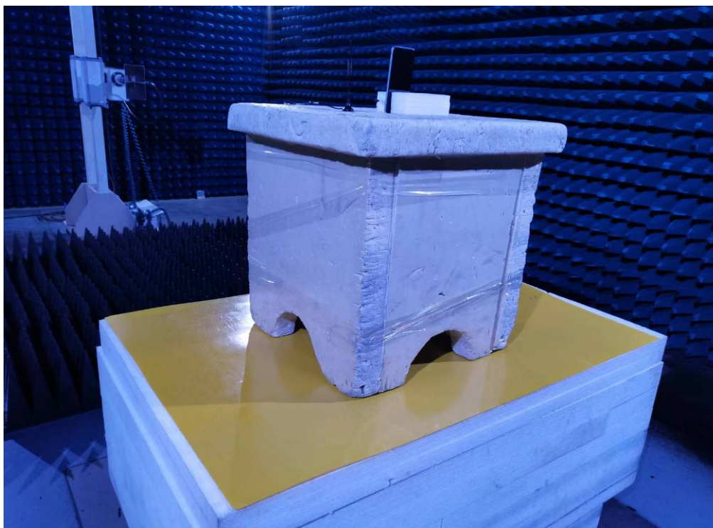
Photo of Radiated Emission Measurement (Above 1G)
