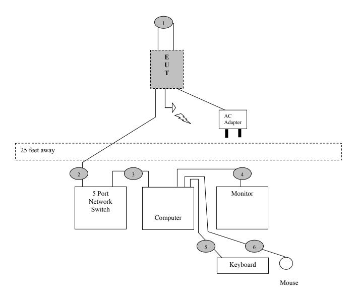
Cable 1: This is a 6-foot braid and foil shielded round cable connecting the EUT's serial port 1 and serial port 2 in loop back configuration. It has metallic DB-9 type connector at both ends. The cable is bundled to a length of one meter and the shield of the cable is grounded to the chassis via the connector shells.
