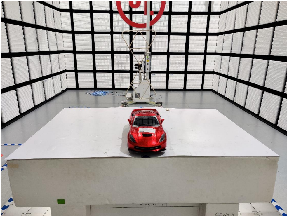
Radiated Emissions above 1GHz test setup photo
